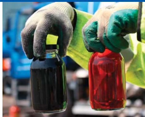
Before and after fuel polishing
